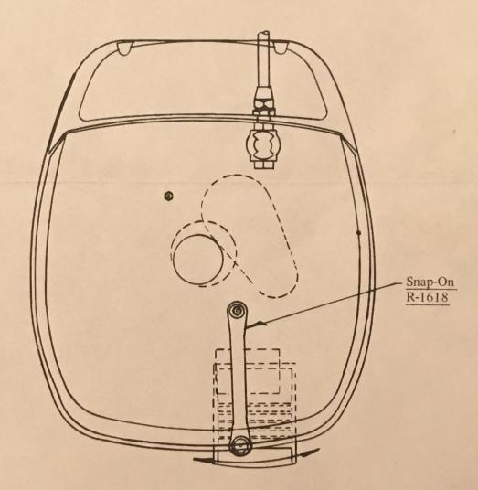
4. Depress pedal and remove the 2 1/2 inch diameter object. Toilet installation is now complete.
