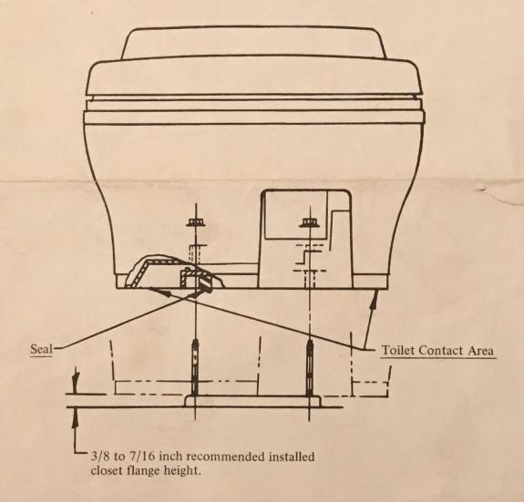
Lay a straight edge across closet flange and measure distance to floor at toilet contact area to check flange installation. Too much gap may cause the flush mechanism to bind. Too little gap may prevent a good seal.
